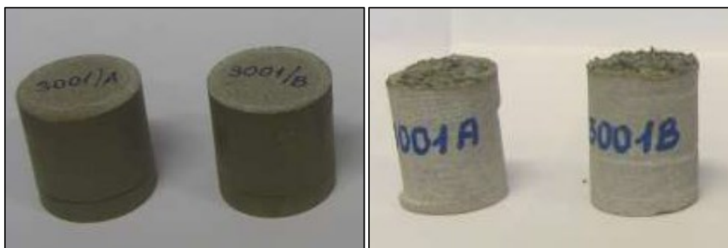
Figure 3. Permeability Test Plug Samples Before and After Laser Treatment
