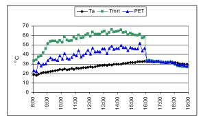
Fig. 3 Daily variation of  $T_a$ ,  $T_{mrt}$  and PET on the Aradi square in Szeged (17<sup>th</sup> August 2006)
