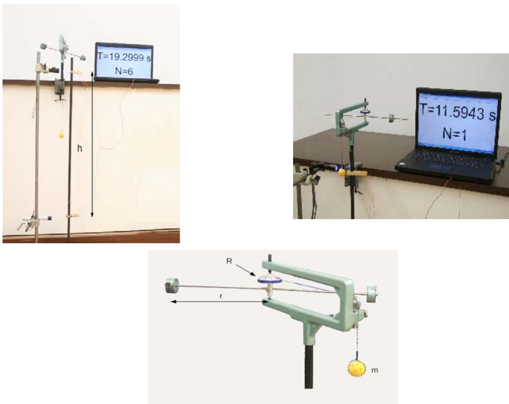
Figure 1. A conventional instrument for demonstrating Newton's second law for rotation
