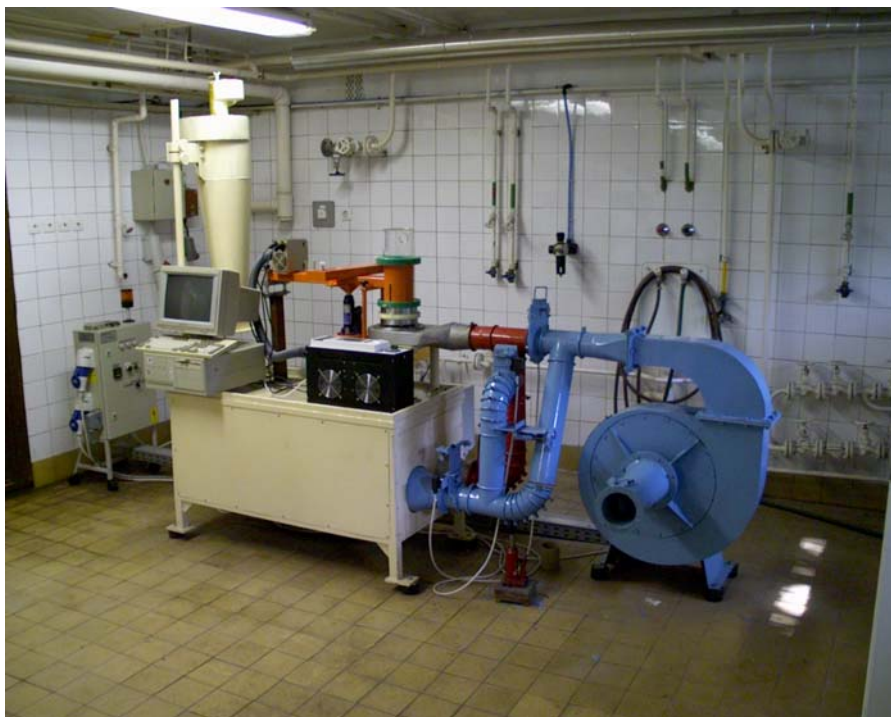
Figure 1. Combined microwave-assisted hot-air vibrofluidised bed experimental drying equipment with homogeneous distribution of electromagnetic field.
