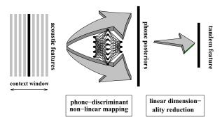
Figure 1: Schematic of phone-based tandem ASR.
