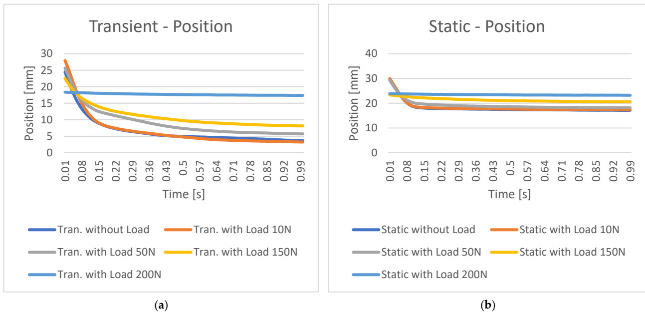
Figure 9. Position measurement results. (a) PAM contraction/time diagram for transient collision; (b) PAM contraction/time diagram for static collision.
