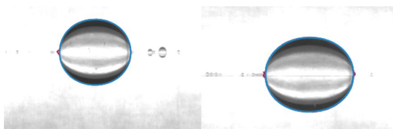
Figure 3. Exported spinning drop instrument picture of the structure of the rapeseed oil droplet in presence of 5.0 g/L aqueous SDS solution after 1.0 min and 15.0 min (droplet volume = 0.35 \mu L).
