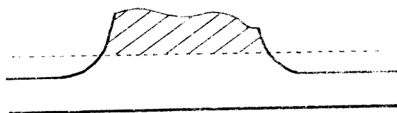
Figure 4.: Peak recording using the constant threshold value.
