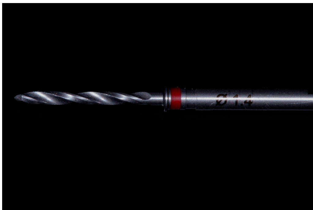
Figure 2. 1.4 mm diameter drill used for the investigation.
