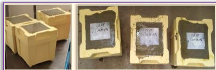
Figure 10. Preparing and labelling the unarmed concrete samples
