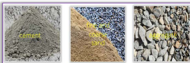
Figure 2. Solid fractions of the concrete recipe
