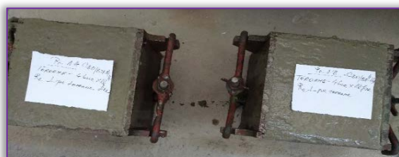
Figure 11. Labelling the reinforced concrete samples of reinforced concrete with recycled polyethylene terephthalate
