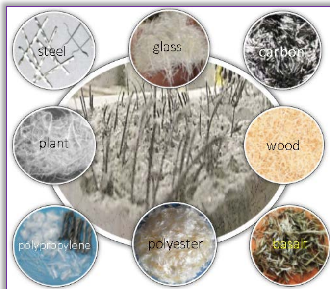
Figure 4. Typically fibers used in fibre–reinforced concretes
