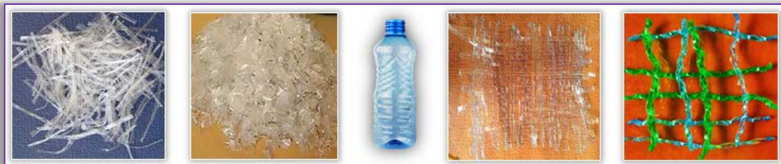
Figure 7. Several reinforcing possibilities with recycled polyethylene terephthalate (PET) (strips, chips, mesh woven and rope strand) [16–18]
