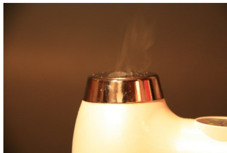
Figure 1. A drop of water on the ultrasound head vibrates, breaking down into tiny particles and forming steam above the head.
