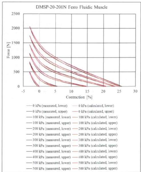
Fig. 7 Approximation of hysteresis loop using (17)
