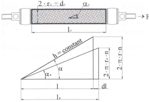
Fig. 2 Geometry parameters of PAMs
