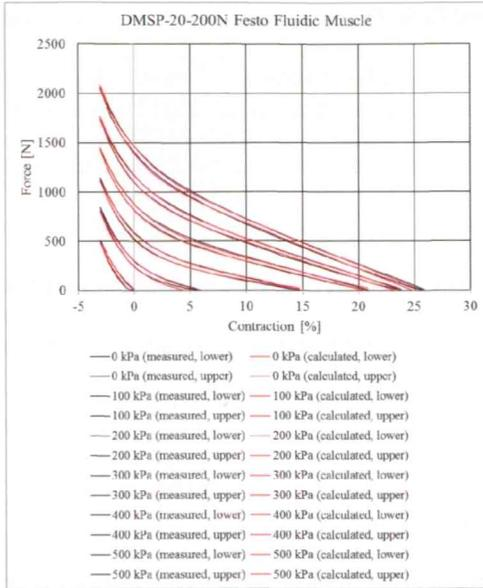
Fig. 8 Approximation of hysteresis loop using (18)
