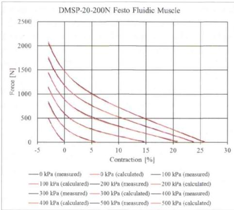
Fig. 5 Comparison of measured data and force model using (18)
