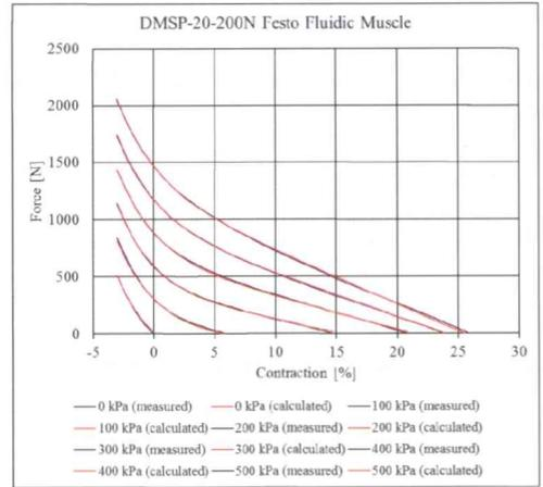
Fig. 4 Comparison of measured data and force model using (17)
