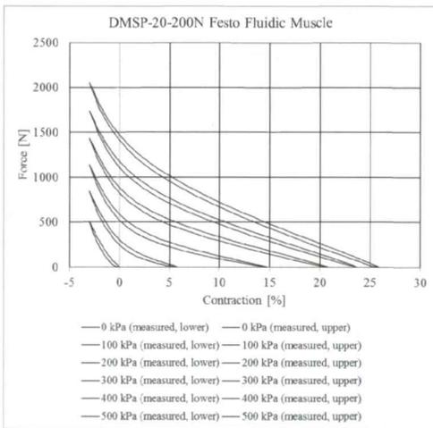
Fig. 6 Hysteresis in the tension-length (contraction) cycle
