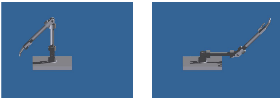
Fig. 2. The VBA Macro program can control this (5 DOF) robot arm by the Angle1 and Angle2 [°] parameters at the shoulder and elbow articulations
