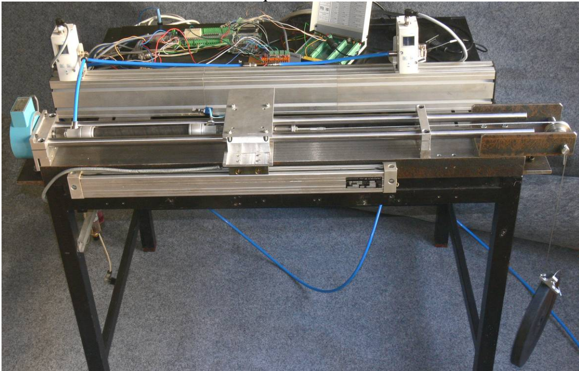
Figure 4. The photo of the stand for Fluidic Muscle investigations in fixed slider position
