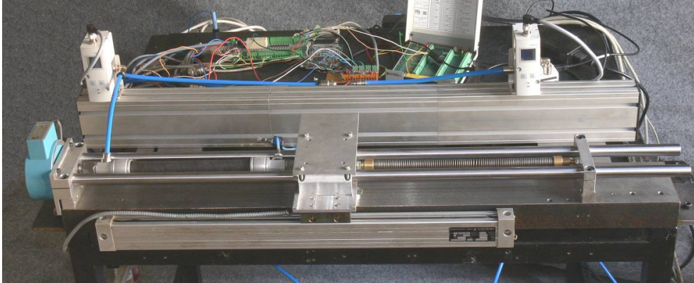
Fig. 7. Experimental set-up for analysis of one muscle and one spring
