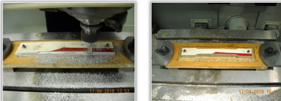
Figure 4. Standard specimen production with milling machine
