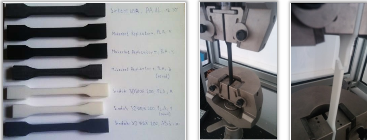
Figure 9. 3D printed specimens with different fibre direction and filling parameters
