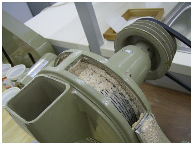
Fig. 7. The perforated plate of SATAKE laboratory machines after the debranning
