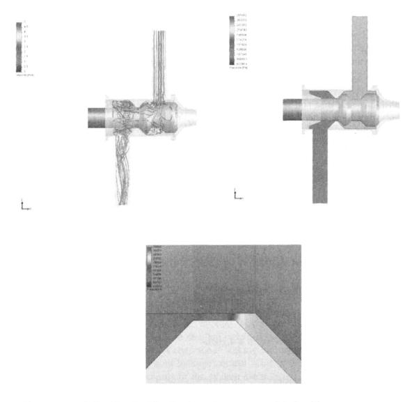
Pressures and liquid velocities in the valve were modeled with computer program. Velocity values evolving in LCFDSV is plotted in the left-hand figure. Liquid pressure values are illustrated in the right-hand side and in the middle figures, respectively.
