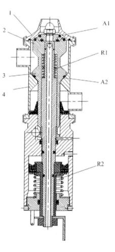
After change the valve is closed at the bottom, an air pressure of 6 bars adds to spring force, so a force  $R_1$  + force originating from air pressure works against  $R_2$ .
